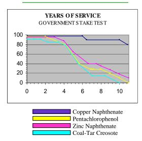
The above data has been accumulated since 1941 for copper naphthenate diluted with a light petroleum solvent.
